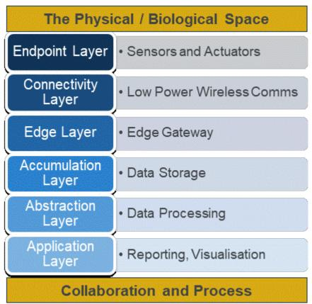
There is typically a layered architecture to an IoT implementation. The endpoint layer is the sensors and actuators embedded in the physical devices (or biological entities).
