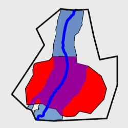
Loss:  $L = SI \times A_f/A_s \times R_D$
