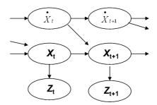
Figure 4.2: Representation of a Kalman filter (depicting a classical situation where both the position  $(x_t)$  and the speed  $(\dot{x}_t)$  of an object are tracked) as a dynamic Bayesian network.
